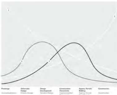
The “MacLeamy Curve” illustrates the concept that decisions made earlier in the design process can be made with greater benefit at less cost (from Integrated Project Delivery: A Guide , © AIA/AIACC, 2007)
